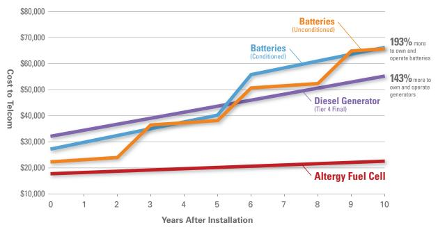
TCO based on a 5kW load, 8 hours of runtime. Battery quantities and size determined at end of battery life. Generators are Tier 4 Final. Analysis includes acquisition costs, plus permitting and installation costs, as well as ongoing maintenance (and battery replacement) costs for all three technology alternatives. Data sources for the analysis include research reports (Batelle, Battery Council International, etc.), Manufacturer data sheets, prices, white papers and Altergy Systems information.
